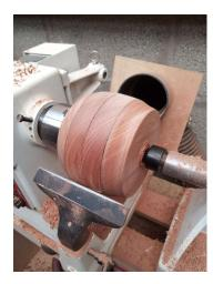
When we have got it roughly round we mount a jacobs chuck on the tailstock and drill another 45mm hole approx 10mm deep so we can turn the box around when we have finished the sides and bottom:
