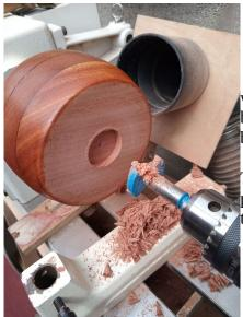
When we have done this we then use a 3.5mm drill bit to drill just into the bottom of the drawer section.
