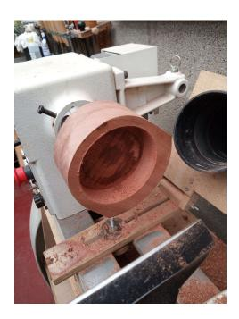
Take extra care with the drawer - as it is not round it will be out of balance on the lathe – start at a slow speed and gradually increase to get a stable suitable turning speed.
